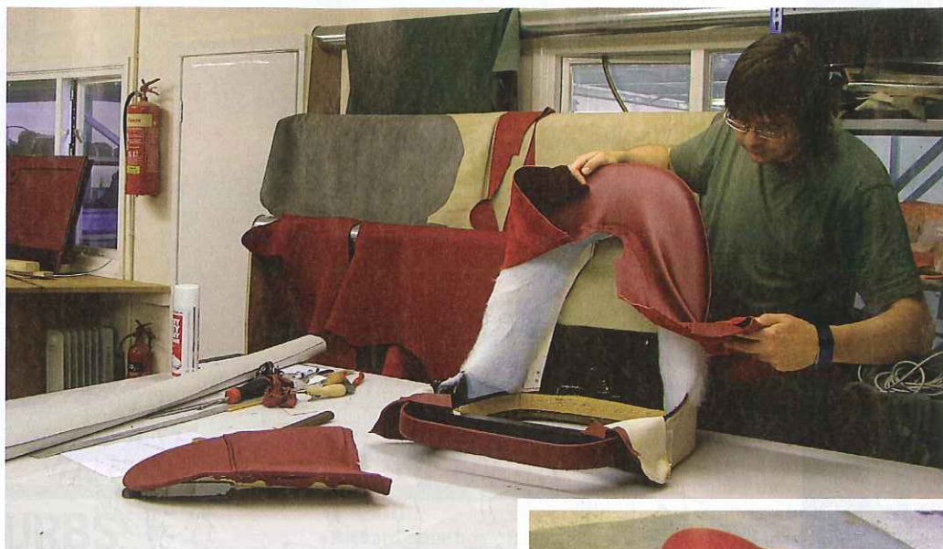
Above: CMC's Tom Hampton gets to work stripping the seat (right). Far right: new seat base (foreground) uses a less bulky base and foam filling (right below). Below: Phil was finally able to get comfortable for the drive to Le Mans
