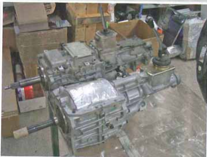
An American 5-speed gearbox for the car.
