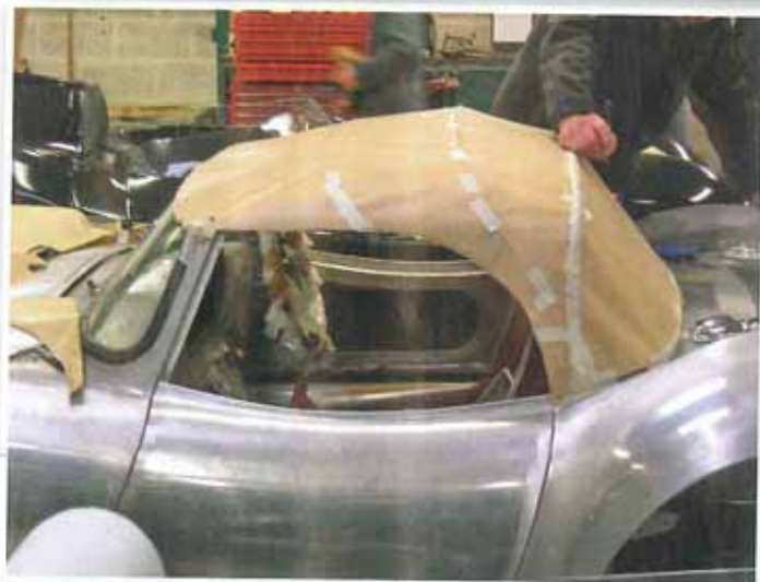
The hood has its origins in an MGB but had to be substantially modified for this purpose and looks quite neat.
