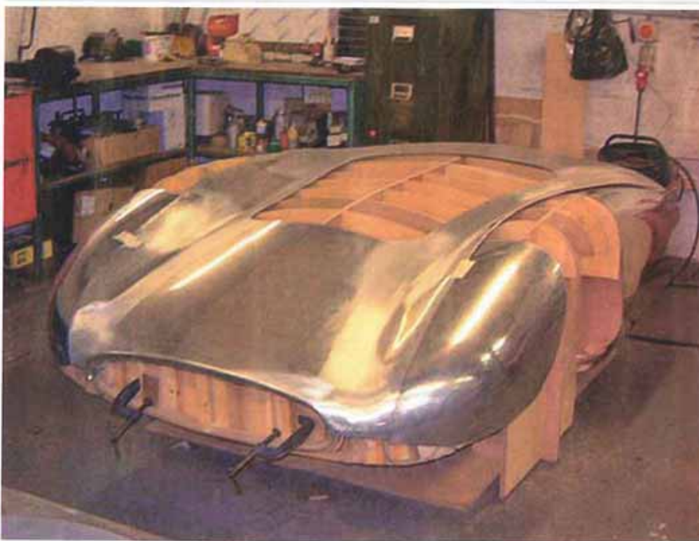
Wooden bucks were made up onto which the individual alloy panels were formed
