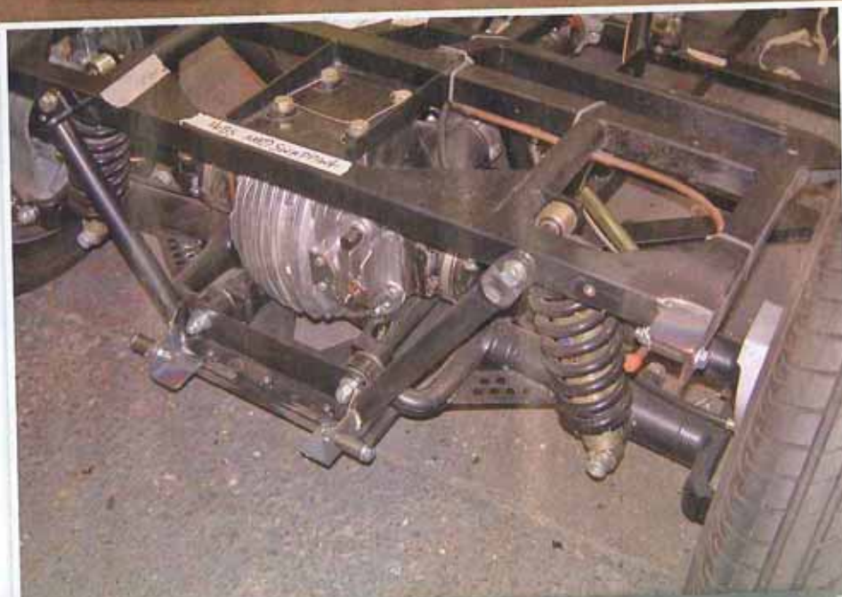
Pretty conventional rear axle/suspension from an XJ40 mounted into the Revival chassis box section.
