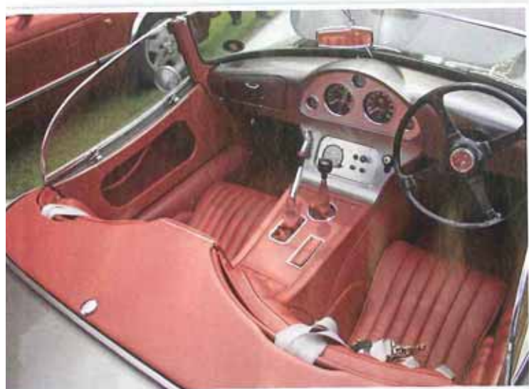
Beautifully hand-crafted and finished leather interior of the car. You can notice a couple of Jaguar items like the specially cut-down XK 4-spoke steering wheel and the leather covered ashtray from a Series saloon. The rear panel behind the seats hinges back to reveal the hood stowage area.
