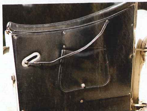
Sidescreens for XK120/140; XK150 got wind-up windows
