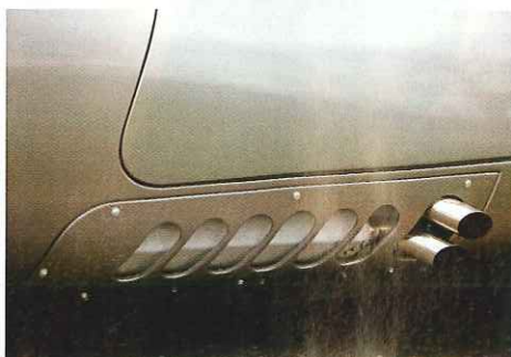
Cooling fins over side-exit exhaust stop passenger baking
