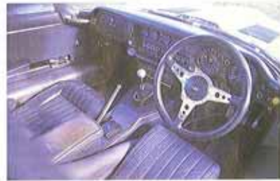
Above: modified E turns in eagerly, then progresses controllably to oversteer. Left: special cams and careful assembly give 4.2-litre straight six 306bhp. Right: racing equipment - bucket seat, kill switch, large oil pressure light - is discreetly blended into original interior
