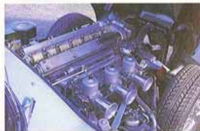
Above: modified E turns in eagerly, then progresses controllably to oversteer. Left: special cams and careful assembly give 4.2-litre straight six 306bhp. Right: racing equipment - bucket seat, kill switch, large oil pressure light - is discreetly blended into original interior
